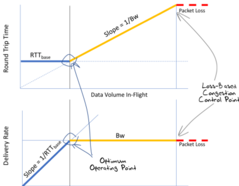
Figure 6 – Delay and Delivery characteristics of a simple Link Model (after [1])
