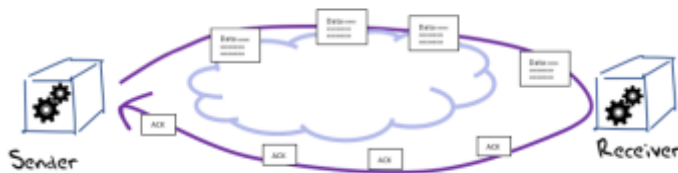
Figure 2 – Ack-pacing flow control
